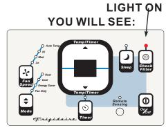
Note: This feature is a reminder to clean the Air Filter (See Care and Cleaning) for more efficient operation and cooling. The LED (light) will illuminate after 250 hours of operation. To reset after cleaning the filter, press the "Clean Filter" button and the light will go off.
